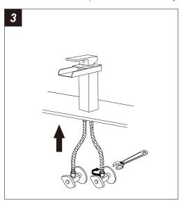
3.Connect the flexible hoses to water supply valve (not included) and copper tubes, and tighten it with adjustable wrench. **DON'T OVER TIGHTEN!**
